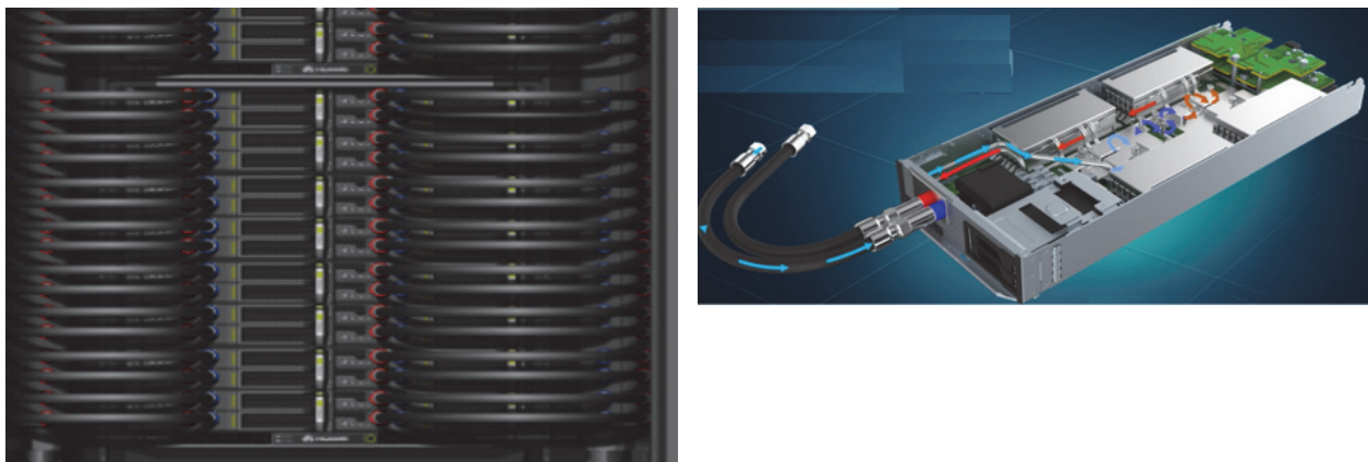
Figure 14 Flexible hose used to connect a manifold to a server blade in a system.
